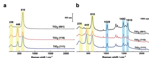
Fig. 2 (a) SHINER spectra of rutile TiO<sub>2</sub>(001), TiO<sub>2</sub>(110), and TiO<sub>2</sub>(111) surfaces in acetonitrile without and (b) with N719 molecules adsorbed.
