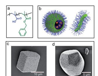
Fig. 1 (a) Generic chemical structure of the PMAA $_{\rm X}$ -PBzMA $_{\rm y}$  diblock copolymer nano-objects used in the study. (b) Schematic representation of PMAA $_{\rm 69}$ -PBzMA $_{\rm 200}$  vesicles and PMAA $_{\rm 71}$ -PBzMA $_{\rm 150}$  worms. (c) SEM images of vesicle/calcite and a (d) worm/calcite composite single crystals.
