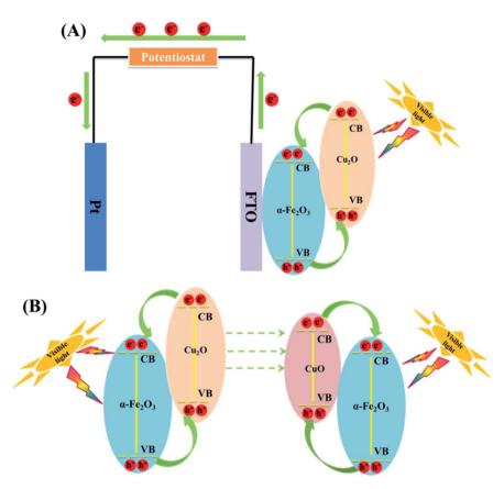
Fig. 4 (A) Schematic diagram of photo-induced electron-hole pairs separated process in PEC system based on  $Cu_2O/\alpha$ -Fe<sub>2</sub>O<sub>3</sub>. (B) A mechanism for the changes of  $Cu_2O/\alpha$ -Fe<sub>2</sub>O<sub>3</sub> after PEC treatment (this figure has been adapted/reproduced from ref. 89 with permission from ELSEVIER, copyright 2018).
