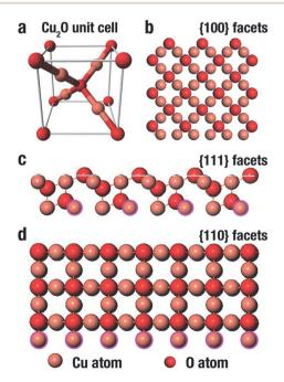
Fig. 3 Representation of the (a)  $Cu_2O$  unit cell, and (b-d)  $Cu_2O$  crystal structure (100), (111) and (110) facet respectively.<sup>74</sup>
