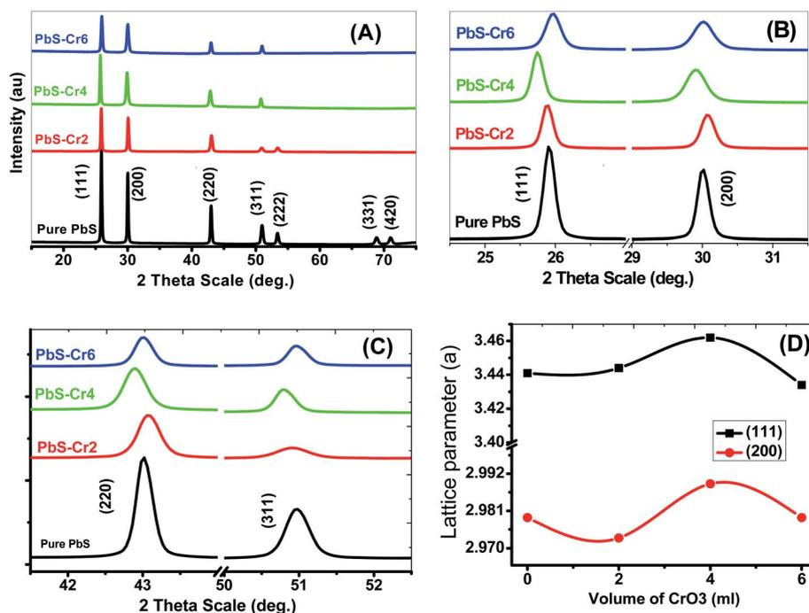
Fig. 1 (A–C) XRD spectra for nanostructure pure and doped PbS thin films with different Cr content. (D) The lattice parameter for (111) and (200) planes.
