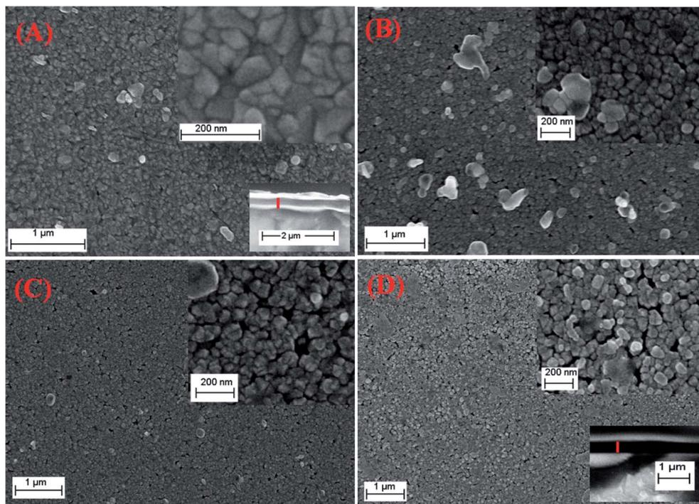
Fig. 3 SEM micrographs for (A) pure PbS, (B) PbS-Cr2, (C) PbS-Cr4 and (D) PbS-Cr6 thin films. The lower insets of (A) and (D) are cross-sectional SEM images.
