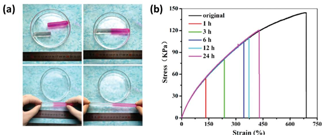
**Fig. 5** (a) Macroscopic self-healing of carbon nanotube-containing hydrogels cut in half and then re-cured at 90 °C. (b) Stress–strain curves of the original and self-healed hydrogel after various healing times. Reprinted (adapted) with permission from ref. 95. Copyright 2017, American Chemical Society.
