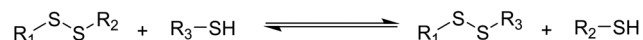
Scheme 3 Formation of disulfide bonds via oxidation of thiols (top) and thiol-disulfide exchange reaction.
