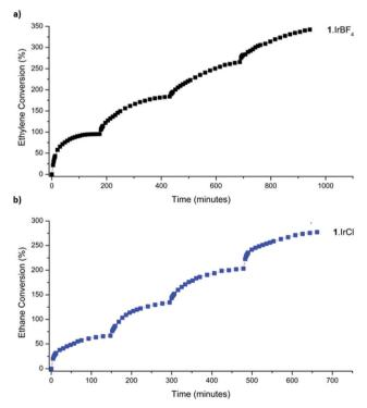
Fig. 3 Catalysis data for the hydrogenation of ethylene at 46  $^{\circ}\text{C}$  (2 bar) using (a) 1-IrBF<sub>4</sub> and (b) 1-IrCl.
