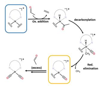
Fig. 2 The proposed mechanism via which mono- and dicarbonyl complexes are generated from decarbonylation of acetaldehyde. The target bis(ethylene) complex 1-IrCl(ETH), and the 1-IrCl(ETH/CO) by product that is also observed, are shown in the blue and yellow boxes. Acetaldehyde can be formed by dehydrogenation of ethanol.
