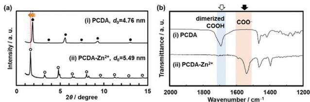
Fig. 8 XRD patterns (a) and FT-IR spectra (b) of the layered PCDA (i) and PCDA-Zn<sup>2+</sup> (ii) samples. Reprinted with permission from Wiley-VCH.<sup>79</sup>
