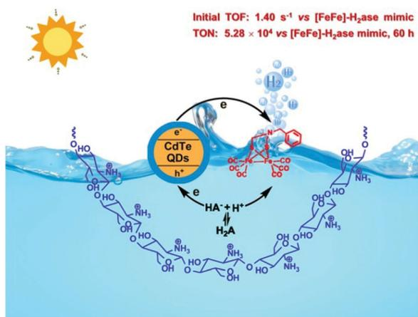
Fig. 7 A schematic describing the H<sub>2</sub> photogeneration of a chitosan-confined mimic of the diiron subsite of [FeFe]-H<sub>2</sub>ase in the presence of CdTe quantum dots and H<sub>2</sub>A. Reprinted with permission from ref. 64. Copyright 2013 Springer Nature.
