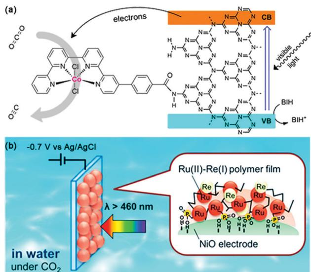
**Fig. 16** (a) Visible-light-driven  $\text{CO}_2$  reduction by a cobalt complex covalently linked to mesoporous carbon nitride. Reprinted with permission from ref. 121. Copyright 2020 American Chemical Society. (b) PolyRuRe/NiO photocathode for  $\text{CO}_2$  photoreduction. Reprinted with permission from ref. 124. Copyright 2019 American Chemical Society.
