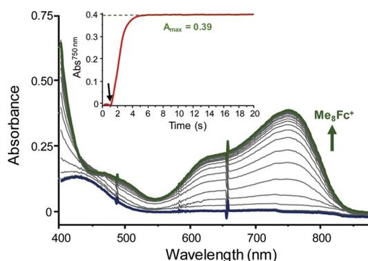
Fig. 2 Representative UV-vis spectra for Me<sub>8</sub>Fc<sup>+</sup> accumulation during ORRs mediated by **1** in air-saturated MeCN at 298 K using **1**/Me<sub>8</sub>Fc/LutHBF<sub>4</sub> at 1/20/400; inset: variation of the Abs<sup>750nm</sup> as a function of time (the green dotted line indicates the theoretical *A*<sub>max</sub> for the total Me<sub>8</sub>Fc conversion); the black arrow indicates the injection of **1**.
