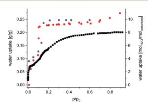
Fig. 2 Gravimetric water adsorption isotherm collected at 298 K for Fe-MIL-59 (red dots), activated at 100 °C and 10<sup>-2</sup> mPa; water content obtained from Rietveld analyses (Table S1.1, ESI†) of PXRD data collected at different relative humidity values at 298 K (blue squares) and water uptake obtained from GCMC simulations (black squares).
