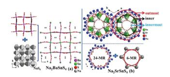
Fig. 2 (a) Crystal structure of  $Na_2BaSnS_4$  along the c-axis: a 3D network composed of edge-sharing  $BaS_8$  dodecahedra, and an edge and corner-sharing  $(NaS_6)_n$  3D network; (b) the whole structure of  $Na_2SrSnS_4$ : three-types of rings (outermost, inner, innermost), 24- $NaS_6$ -MR, and 6- $SrS_7$ -MR.
