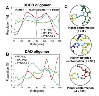
Fig. 4 Distributions of the torsional angle between (A) the donor and bridge on the DBDB oligomers, and between (B) the donor and acceptor on the DAD oligomers; (C) the representative planar conformations ( $\theta \sim 0^{\circ}$  or  $\sim 180^{\circ}$ ) and highly distorted conformation ( $\theta$  $\sim$ 90°), where the torsional angles are marked in light blue color and hydrogen atoms are not shown for clarity.
