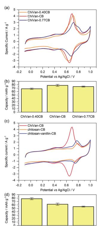
Fig. 4 (a and c) Cyclic voltammetry and (b and d) average capacities as calculated by integration of the cyclic voltammetry curves of ChiVan–carbon black composites prepared with different ratios of both constituents (a and b) or composites of carbon black with ChiVan or other polymers in which certain steps of the ChiVan synthesis were omitted (c and d). All CV was tested in 1 M HClO<sub>4</sub> aqueous solution (5 mV s $^{-1}$ ). The fifth cycle of the respective experiment is displayed.
