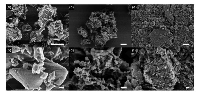
Fig. 3 SEM images of carbon black (a and b) and ChiVan–CB before (c and d) and after (e and f) grinding. The scale bars represent 6 μm (a, c, and e) and 600 nm (b, d, and f), respectively.
