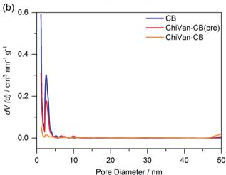
Fig. 2 Nitrogen sorption measurement of carbon black (blue), a ChiVan–CB mixture (red), and ChiVan–CB after grinding (orange). (a) Isotherms and (b) pore size distribution.
