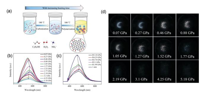
Fig. 5 (a) Schematic of the facile synthesis of N-CDs via a one-step ethanol-thermal strategy treated with H<sub>2</sub>O<sub>2</sub> and NH<sub>3</sub>·H<sub>2</sub>O. (b) PL spectra of N-CDs with increasing pressure. (c) PL spectra of N-CDs as the pressure decreases to ambient conditions. (d) Optical photographs of N-CDs with increasing pressure. Reproduced with permission from ref. 43. Copyright 2018 American Chemical Society.
