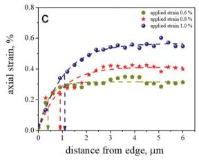
Fig. 4 Optical micrograph of the fully embedded 1LG ribbon obtained *via* direct exfoliation on the PMMA bar and consequent spin coating (a). The distribution of  $\omega_{2D}$  along the mapping line at the left-hand end of the ribbon at rest highlights an initial non-uniform, compressive, strain distribution (b); axial strain profiles for three strain levels derived from the Raman wavenumber distributions of 2D peaks (c).
