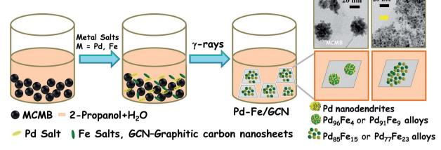
Scheme 1 Schematic illustration of radiochemical synthesis of the Pd-Fe bimetallic alloy on carbon nanosheets.
