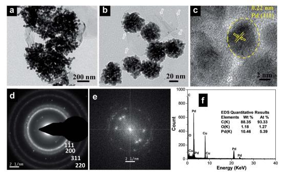
Fig. 1 (a and b) Transmission electron micrographs of the  $Pd_{100}$ /GCN nanohybrid at two different magnifications, (c) HRTEM image of palladium nanoparticles, (d) SAED pattern and (e) FFT and (f) EDS spectrum of the  $Pd_{100}$ /GCN nanohybrid. The white arrows represent the thin sheets of graphitic carbon.
