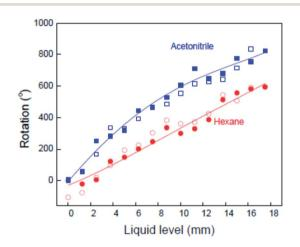
Fig. 10 The observed dependence of the paddle rotation angle on the yarn immersion depth in acetonitrile and in hexane for an 8  $\mu$ m diameter, neat MWNT yarn having 25 000 turns per m of inserted twist. Closed and open symbols are for liquid filling and removal, respectively. The lines are a guide to the eye. This figure has been reproduced from ref. 4 with permission from AAAS.
