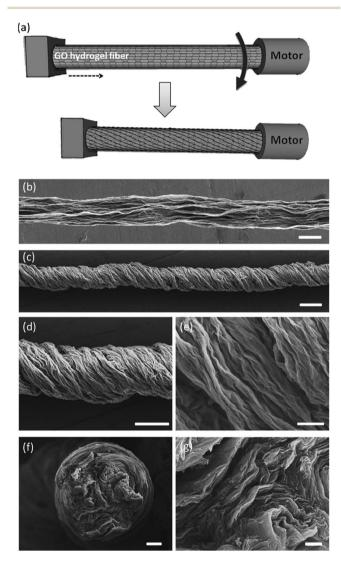
Fabrication and characterization of graphene fiber artificial muscles, (a) scheme of the graphene fiber fabrication; the arrow indicates the direction of rotation; (b and c) SEM images of the directly dried graphene fiber and twisted graphene fiber; (d and e) enlarged view of the twisted graphene fiber and its surface respectively; (f) cross-section of a graphene fiber; (g) enlarged cross-section of the graphene fiber. This figure has been reproduced from ref. 11 with permission from Wiley-VCH.
