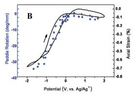
Fig. 13 Electrochemical torsional and tensile actuation for two-end-tethered, neat MWNT yarns half immersed in liquid electrolyte. Yarns were either prepared as S twist (A) or Z twist (B). Negative paddle rotations indicate rotation in the untwist direction and negative strains indicate length contraction. This figure has been reproduced from ref. 3 with permission from AAAS.
