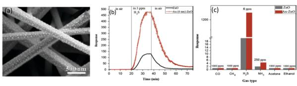
Fig. 16 (a) SEM image of Au/ZnO nanorods; (b) response/recovery curves of the Au/ZnO nanorod-based sensor and pristine ZnO nanorod-based sensor to 3 ppm H<sub>2</sub>S at room temperature; (c) responses of the Au/ZnO nanorod-based sensor and pure ZnO nanorod-based sensor to different gases.<sup>257</sup> Copyright 2015, Elsevier.
