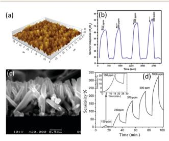
Fig. 8 (a) AFM image of the ZnO films and (b) response/recovery curves of a ZnO film-based gas sensor to different concentrations of H<sub>2</sub>. <sup>189</sup> Copyright 2014, Springer Nature. (c) Cross section SEM image of the ZnO nanorods and (d) response/recovery curves of a ZnO nanorodbased gas sensor to different concentrations of H<sub>2</sub>. 191 Copyright 2013, Elsevier.
