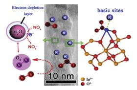
Fig. 22 Gas sensing mechanism to  $NO_x$  of mesoporous  $K_2O-In_2O_3$ nanowires. 129 Copyright 2016, Elsevier.
