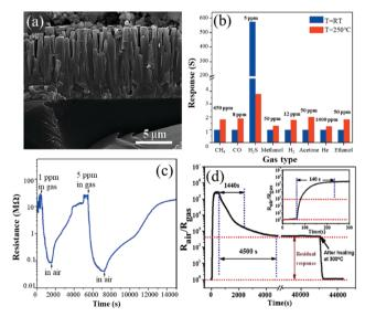
Fig. 4 (a) Cross-section SEM image of vertically aligned ZnO rods; (b) selectivity of the sensor at 25 °C and 250 °C; (c) response/recovery curves to 1 and 5 ppm  $H_2S$  at room temperature. Copyright 2015, Elsevier. (d) The response/recovery curve at 50 ppm  $H_2S$  gas at room temperature. Copyright 2017, Elsevier.
