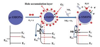
$E_C$ : bottom of conduction band;  $E_V$ : top of valence band;  $E_{Fn}$ : bulk Fermi level;  $\mathbf{E}_{Fs}$ : surface Fermi level;  $\Delta \varphi$ : potential barrier;
