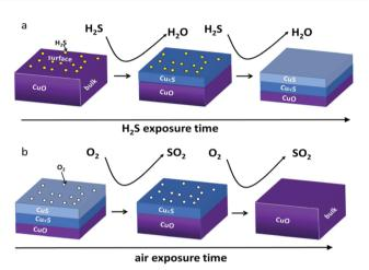
Fig. 11 Schematic diagrams of the sensing mechanism of CuO: (a) response process in H<sub>2</sub>S and (b) recovery process in air. <sup>93</sup> Copyright 2016, American Chemical Society
