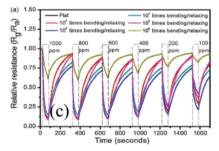
Fig. 26 (a) SEM images of Pd/ZnO nanorods after  $10^3$  times bending/relaxing. (b) Response/recovery curves of the flexible sensor to  $H_2$  at different bending angles, (c) the reliability test of the flexible sensor. <sup>173</sup> Copyright 2013, Elsevier.
