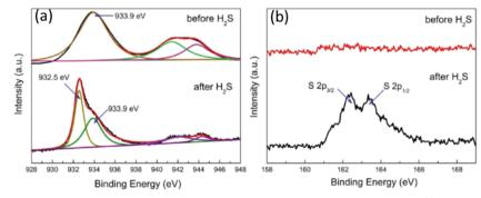
Fig. 12 (a) Cu 2p<sub>3/2</sub> and (b) S 2p XPS spectra of porous CuO nanosheets before and after exposure to H<sub>2</sub>S. 93 Copyright 2016, American Chemical Society
