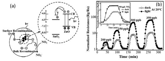
Fig. 25 (a) Schematic diagram of the carrier transport under UV light and the electron-hole pair separation on heterostructure of ZnO/SnO<sub>2</sub> composite; (b) response/recovery of ZnO/SnO<sub>2</sub> composites at different concentrations of NO<sub>2</sub> with and without UV light stimulation at room temperature.<sup>395</sup> Copyright 2011, Elsevier.
