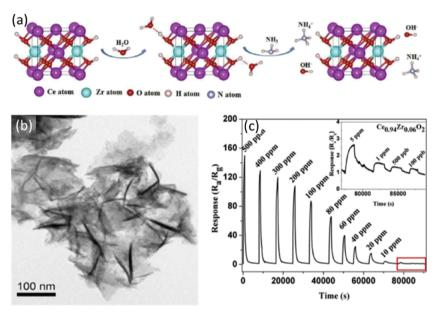
Fig. 18 (a) Schematic diagrams of the NH<sub>3</sub> reaction mechanism on the surface of  $Ce_{0.94}Zr_{0.06}O_2$  nano-sheets; (b) TEM image of porous  $Ce_{0.94}Zr_{0.06}O_2$ nano-sheets; (c) response/recovery curves of the porous  $Ce_{0.94}Zr_{0.06}O_2$  nanosheet based sensor to NH<sub>3</sub>. <sup>127</sup> Copyright 2018, Elsevier.
