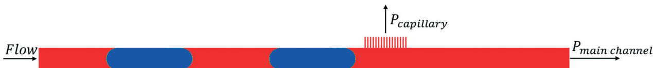
Fig. 2 Scheme of the simplified CFD simulation setup of the capillary separator.
