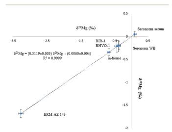
Fig. 2 Bivariate Mg isotope ratio plot (or 3-isotope plot) for standards, biological and geological reference materials.  $\delta$ Mg values are expressed relative to the DSM3 isotopic reference material.
