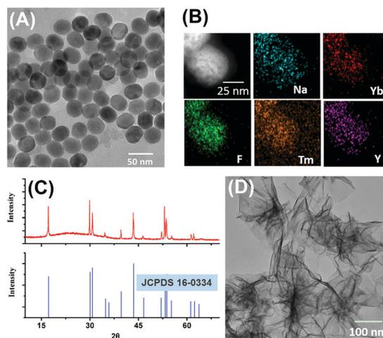
**Fig. 1** TEM (A), EDS mapping (B) and X-ray diffraction (XRD) patterns (C) of NaYF<sub>4</sub>:Yb,Tm UCNP; (D) TEM of MnO<sub>2</sub> nanosheets.
