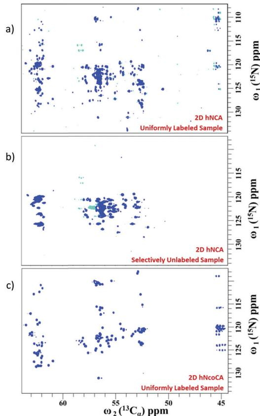
Fig. 3 (a) The complete 2D hNCA spectrum of the uniformly labeled sample, (b) 2D hNCA of selectively unlabeled sample and (c) 2D hNCoCA spectrum of the uniformly labeled sample. Note that in this approach, the 2D hNCoCA spectrum of the selectively unlabeled sample is not needed (see text).
