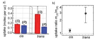
Fig. 4 Enantioselective adsorption. (a) Uptake of (*S*)-phenylethanol  $m_{(S)}$  and (*R*)-phenylethanol  $m_{(R)}$  by the homochiral SURMOF in the *trans* and *cis* state. (b) Ratio of  $m_{(S)}$  and  $m_{(R)}$  for the sample in the *trans* and *cis* states with the standard deviation as error bars.
