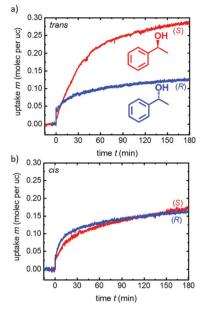
Fig. 3 Enantiopure uptakes of (R)- and (S)-phenylethanol by the  $Cu_2(DCam)_2(AzoBiPyB)$  film in the trans state (a) and cis state (b). The uptake is determined with a quartz crystal microbalance (QCM) in combination with a gas flow system. The molecular structures of (R)- and (S)-phenylethanol are sketched in the inset in (a).
