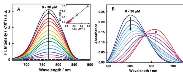
**Fig. 1** (A) Fluorescence spectra of  $15 \mu\text{M}$  styryl-11 with increasing concentration of insulin fibrils ( $0$ – $30 \mu\text{M}$ ) [ $\lambda_{\text{ex}} = 630$  nm]. Inset shows the double reciprocal plot ( $1/F$  vs.  $1/C$ ) and the solid line represents the fitting of the data points according to the  $1:1$  binding model. (B) Absorption spectra of  $15 \mu\text{M}$  styryl-11 with the increase in concentration of insulin fibrils ( $0$ – $30 \mu\text{M}$ ).
