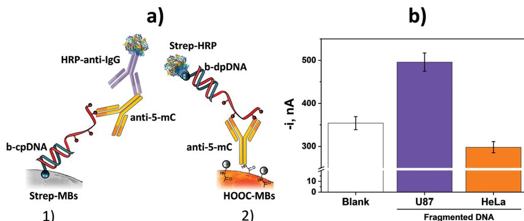
**Fig. 12** (a) Schematic illustration of strategies developed for the PCR-free determination of 5-mCs in DNA (DNA sensor, 1, and immuno-DNA sensor, 2), and (b) amperometric responses provided by the DNA sensor in the absence of target DNA (blank) and in the presence of 100 ng of genomic DNA extracted and fragmented with ultrasound from U87 and HeLa cells. Error bars are three times the standard deviation of three replicates. Reproduced and adapted from ref. 27 and 28 with permission.
