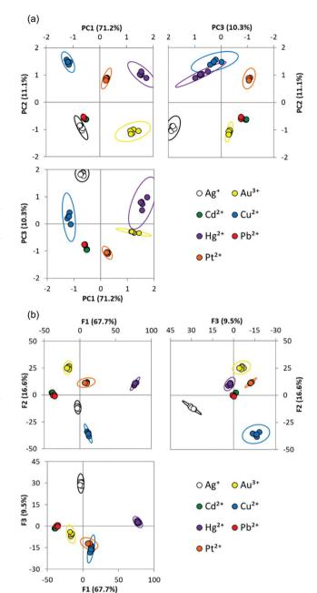
Fig. 2 (a) PCA score plot for the analysis of seven metal ions (confidence ellipsoids at 95% probability) performed in quintuplicate (1 mM metal ion, pH 7.4, 20 mM HEPES) describing the response to thiocoumarin 545 in eight solvents. (b) LDA score plot of the same data, with 95% confidence ellipsoids. In each analysis, each pairing of the three main factors is plotted in a separate 2D plot.
