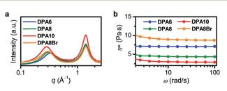
Fig. 3 (a) SWAXS profiles and (b) complex viscosity ( $\eta^*$ ) of DPA6 (blue), DPA8 (green), DPA10 (red), and DPA8Br (orange) at 30 °C (ω, angular frequency).
