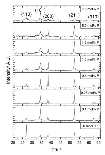
Fig. 2 X-ray diffraction patterns for P:SnO<sub>2</sub> thin films deposited by AACVD at 550 °C. A change in preferred orientation is observed between undoped, and inclusion of phosphorus into the crystal structure.
