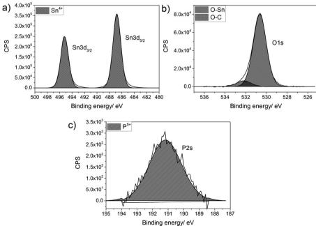
Fig. 1 Typical X-ray photoelectron spectra for (a) Sn 3d environment, (b) O 1s environment and (c) P 2s environment for P-doped SnO<sub>2</sub> films
