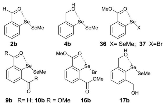
It is noteworthy that the 2-substituted systems show shorter chalcogen bonds with more linear O $\cdots$ Se-X angles than the corresponding 2,6-disubstituted systems indicating the
