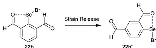
Fig. 15 An example of transforming the 2,6-disubstituted system into its 2,4-disubstituted isomer.
