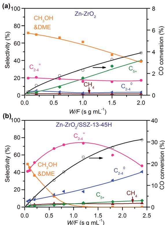
Fig. 8 Effect of contact time on catalytic behaviours of Zn-ZrO<sub>2</sub> and Zn-ZrO<sub>2</sub>/SSZ-13-45H catalysts. Reaction conditions:  $W(\text{Zn-ZrO}_2) = 0.030\text{--}1.0$  g;  $W(\text{Zn-ZrO}_2/\text{SSZ-13-45H}) = 0.030\text{--}1.2$  g;  $\text{H}_2/\text{CO} = 2/1$ ;  $P = 3$  MPa;  $T = 673$  K;  $F = 30$  mL min<sup>-1</sup>; time on stream, 10 h.
