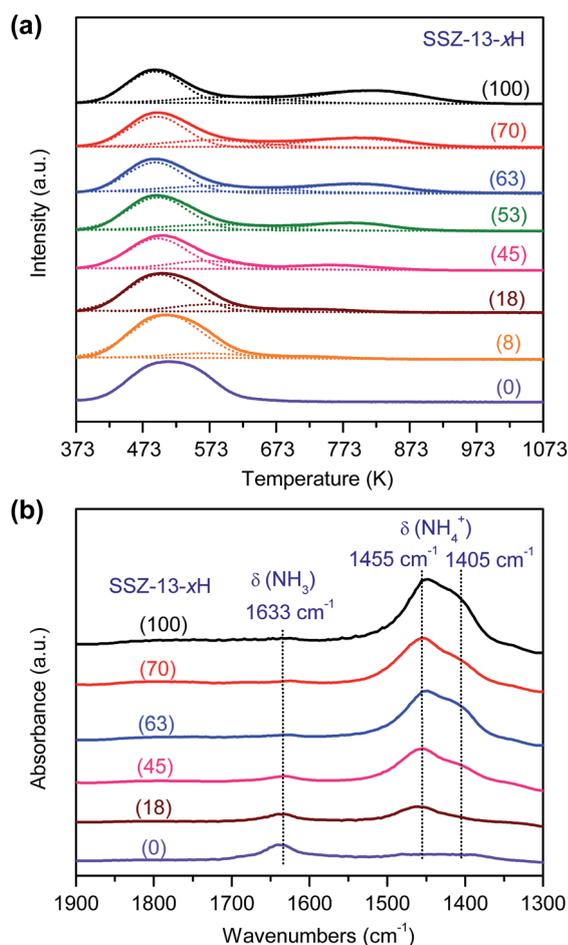
Fig. 4 Characterization of acidity of SSZ-13 with different H<sup>+</sup>-exchanging degrees. (a) NH<sub>3</sub>-TPD profiles. (b) NH<sub>3</sub>-adsorbed FT-IR spectra. The number in the parentheses after each sample denotes the H<sup>+</sup>-exchanging degree.
