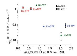
Fig. 6 Relationship between  $\Delta G$  (COOH\*) at 0 V and  $j_{\rm co}$  at -0.9 V. The error bar represents the standard deviation from three experimental trial
