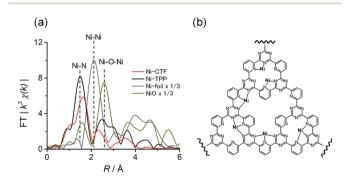
Fig. 1 (a) The  $k^3$ -weighted Fourier transform EXAFS spectra at the Ni K-edge of Ni-CTF (red), Ni-TPP (black), Ni foil (gray) and NiO (dark yellow), and (b) an illustration showing the Ni sites in Ni-CTF (weakly adsorbed molecules in electrolyte, such as water and ethanol used for the preparation of electrode, are not shown for clarity).
