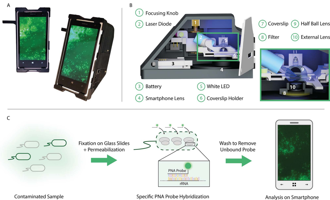
Fig. 1 Selective targeting and imaging of single bacteria on a smartphone. (A) Photographs of a smartphone microscope displaying images of fluorescently labeled Cronobacter spp. bacteria. (B) 3D illustration of the same optomechanical unit that is mounted on the smartphone in (A). (C) Schematic illustration of the bacterial detection procedure. Bacteria from the contaminated sample are fixed on 22 \times 50 mm 2 glass slides and the bacterial membrane is permeabilized in order for the PNA probe to enter the bacteria. An Alexa Fluor 488 dye is chemically linked to the PNA probe which in turn is designed to bind specifically to certain regions of the ribosomal RNA (rRNA) of the bacteria. After washing away unbound probes, only the targeted bacteria remain fluorescent and can be imaged using the smartphone-based microscope shown in (A).
