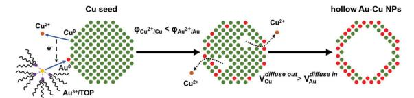
Scheme 1 Growth mechanism of hollow Au-Cu NPs.
