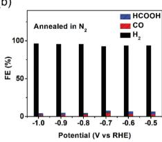
potential-dependent FEs for Fig. 5 Reduction electrochemical reduction of CO<sub>2</sub> at different potentials measured on hollow Au-Cu NP/ C annealed in  $O_2$  (a) and  $N_2$  (b).
