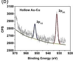
Fig. 2 PXRD pattern (a) and Cu 2p XPS spectrum (b) of hollow Au-Cu NP/C.
