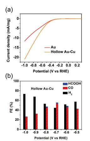
Fig. 3 LSV curves of Au NP/C and hollow Au-Cu NP/C in the CO<sub>2</sub>saturated 0.5 M KHCO<sub>3</sub> at a scan rate of 5 mV s<sup>-1</sup> (a); FEs of various products at different potentials measured on hollow Au-Cu NP/C (b). The current density of different catalysts was normalized with reference to the mass of gold they each contained.
