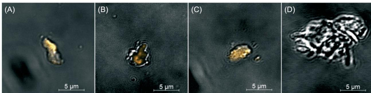
Fig. 6 CLSM images of fragments released from CdSe/ZnS-PMMA (A–C) and PMMA (D) after one day of UVC irradiation, where orange indicates any emission detected above 505 nm.
