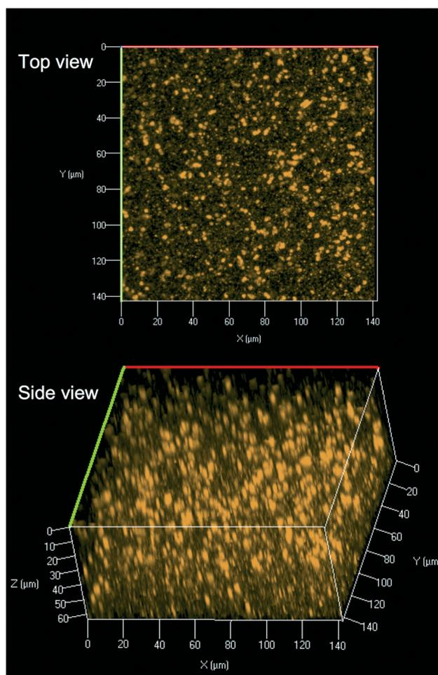
Fig. 2  $142.86\ \mu\text{m} \times 142.86\ \mu\text{m}$  CLSM  $64\ \mu\text{m}$  Z-stack image of CdSe/ZnS-PMMA polymer nanocomposite obtained with 458 nm excitation. Any emission detected above a 505 nm cut-off filter is shown in orange, which includes the QD  $\lambda_{\text{max}} = 594\ \text{nm}$ .
