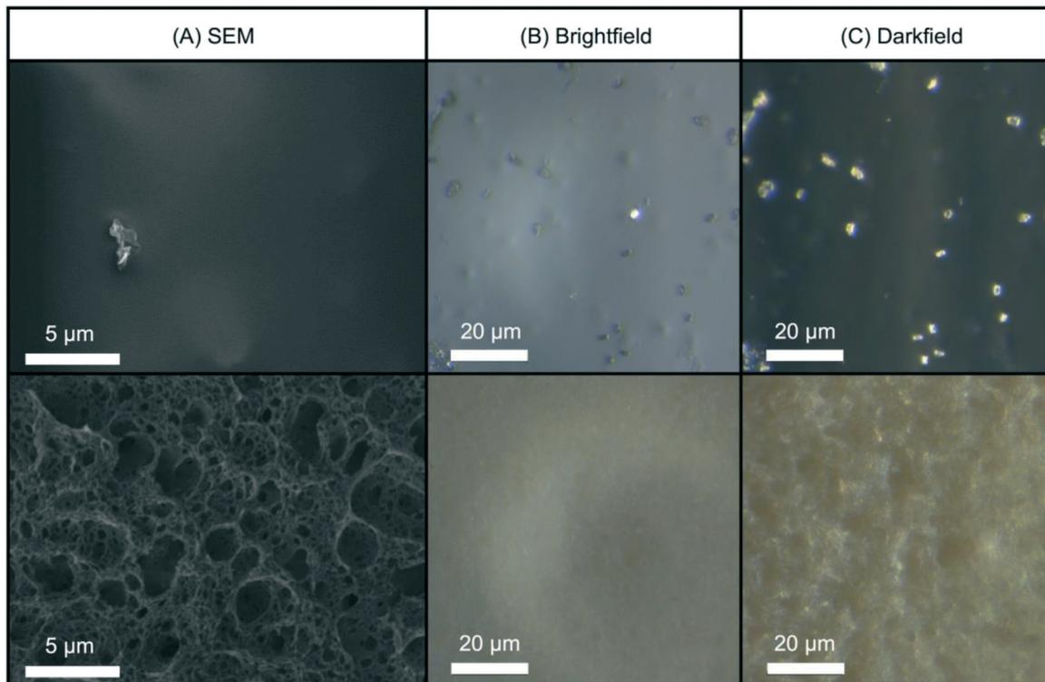
Fig. 3 (A) SEM, (B) bright-field, and (C) dark-field images of the CdSe/ZnS-PMMA nanocomposite surface before (top) and after (bottom) three weeks of UVC irradiation.
