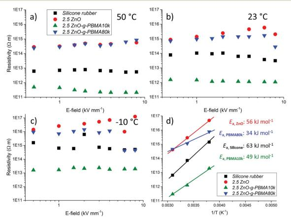
Fig. 14 Resistivity data for silicone rubber, 2.5ZnO, 2.5ZnO-g-PBMA10k and 2.5ZnO-g-PBMA80k at (a) 50 °C, (b) 23 °C and (c) -10 °C. (d) The logarithmic average resistivity plotted against 1/T. Curve fitting gives the slopes corresponding to the temperature dependence of the resistivity and the activation energy of the materials.
