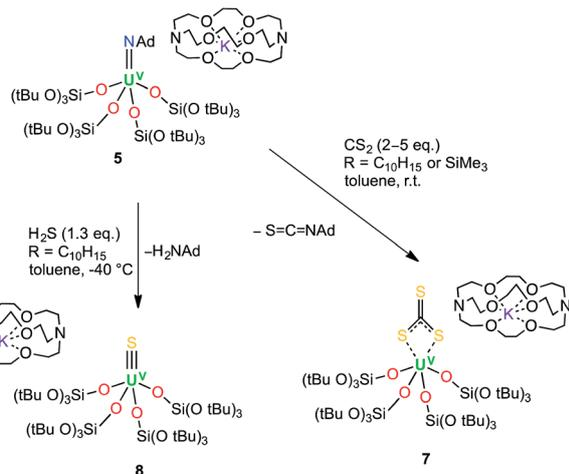
Scheme 3 Syntheses of the terminal U<sup>V</sup> trithiocarbonate complex, [K(2.2.2-cryptand)][U(CS<sub>3</sub>){OSi(OtBu)<sub>3</sub>]<sub>4</sub>] (**7**), and the terminal U<sup>V</sup> sulfide complex, [K(2.2.2-cryptand)][US(OSi(OtBu)<sub>3</sub>)]<sub>4</sub>] (**8**).
