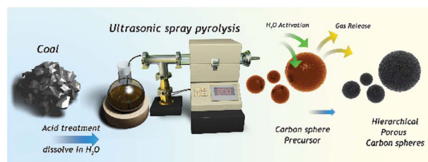
Scheme 1 Schematic diagram of the formation of coal based hierarchical porous carbon spheres.
