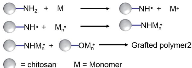
Fig. 3 Grafting mechanism of chitosan under microwave irradiation. Reproduced from ref. 60. Copyright (2004), with permission from Wiley-VCH.
