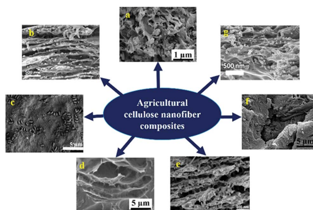
Fig. 5 SEM images of various nanocomposites delivered using plant CNF (a) softwood derived CNF and PLA blend 110 (b) core shell nanofiber obtained by blending spruce sulphite pulp derived CNF and amylopectin (c) soft wood sulphite pulp derived nanofibrillated cellulose–HEC composite 119 (d) palm tree ranchis processed CNF and polyurethane blend 172 (e) Core–shell image of hemicellulose and spruce sulphite pulp extracted CNF blend 171 (f) Pinus sp. and Eucalyptus sp. extracted cellulose nanofiber–polyester blend 173 (g) composite obtained from 1-butyl-3-methylimidazolium chloride (BMIMCl) and canola straw derived CNF 174 (all images were reproduced with permission).
