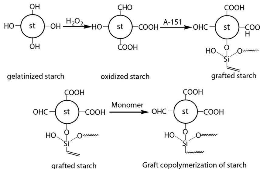
Fig. 16 Reaction pathway for the synthesis of starch-based adhesive (reproduced from ref. 155 with permission from Elsevier Ltd).
