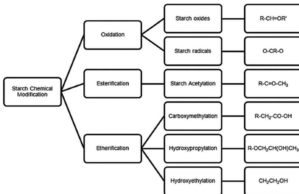
Fig. 9 Schematic summarizing classical chemical methods for starch modification (reproduced from ref. 67 with permission from Elsevier Ltd).
