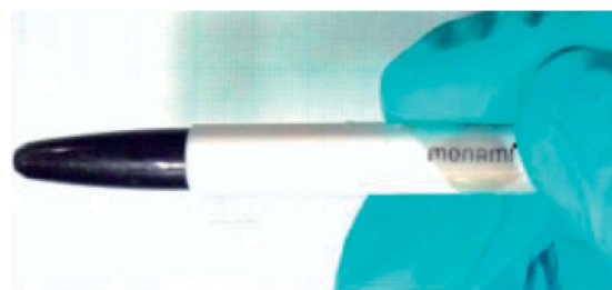
Fig. 22 Fully rollable graphene-based NG. 103
