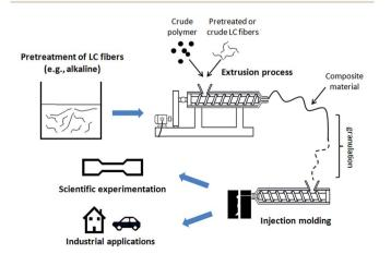
Fig. 5 Pretreatment of LC fibers and their incorporation into a polymeric matrix by extrusion process prior injection molding.
