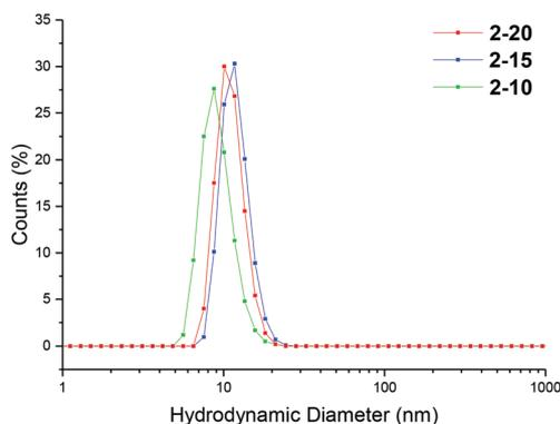
**Fig. 2** Size distributions, by number, for PEGA armed particles 2-20, 2-15, 2-10, obtained by DLS (detection angle = 173°) at 5 mg mL<sup>-1</sup> carried out in chloroform at 25 °C.
