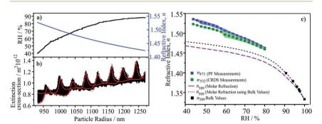
Fig. 5 (a) Relative humidity and refractive index variations as a function of the size of an evaporating Mixture 1 solution droplet. (b) Extinction cross-section (black dots) from measured cavity ring-down times for the same droplet as in panel (a), together with Mie theory calculations (red lines). (c) Wavelength dependence of  $n\text{-RI}\ vs.$  RH for Mixture 1 (measurements are averaged over 3 droplet measurements, envelope shows standard deviation).
