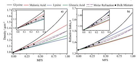
Fig. 1 Density (a) and refractive index (b) parameterisations as a function of solute mass fraction in binary solutions of the four organic components in Mixture 1 (solid lines).<sup>72</sup> Calculations for Mixture 1 from the single components properties (purple dashed line) and from the fitting (black dotted line) of measured bulk data (squares) are also shown.
