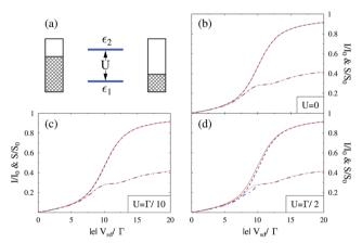
Fig. 13 Full counting statistics of electron transport in junctions. Simulation is performed for Hubbard model (a),  $\hat{H}_M = \sum_{i=1,2} \varepsilon_i \hat{n}_i + U \hat{n}_1 \hat{n}_2$ ,
