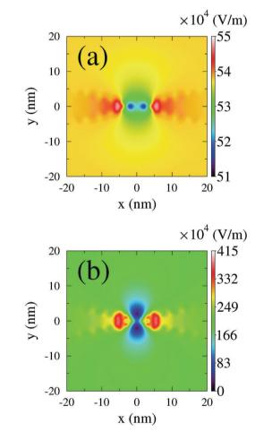
Fig. 5 Instantaneous near field strength in a junction calculated (a) without and (b) with the molecular response. Reprinted (figure) with permission from [A. J. White, M. Sukharev, and M. Galperin, Phys. Rev. B: Condens. Matter Mater. Phys., 2012, 86, 205324.] Copyright (2012) by the American Physical Society. http://dx.doi.org/10.1103/PhysRevB.86.205324.
