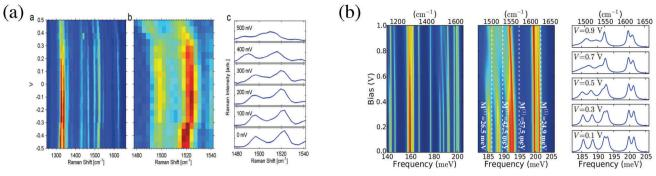
Fig. 8 Bias dependence of Raman shift in OPV3 junction. Shown are (a) experimental data and (b) a theoretical analysis. (a) Reprinted with permission from Macmillan Publishers Ltd: [Nat. Nanotechnol.] (ref. 96), Copyright (2011). (b) Reprinted with permission from [K. Kaasbjerg, T. Novotný, and A. Nitzan, Phys. Rev. B: Condens. Matter Mater. Phys., 2013, 88, 201405.] Copyright (2013) by the American Physical Society. http://dx.doi.org/10.1103/PhysRevB.88.201405
