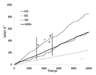
**Fig. 10** MSD plot in all directions of an individual isobutane molecule in silicalite-1 at 450 K. Each symbol signifies the assigned portion of the trajectory plot shown in Fig. 11. Reproduced from ref. 59 with permission from the American Chemical Society.
