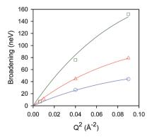
Fig. 8 Broadenings obtained for isobutane in silicalite-1 at: 444 K ( $\bigcirc$ ), 491 K ( $\triangle$ ), and 550 K ( $\square$ ). The solid lines correspond to a Chudley–Elliot jump diffusion model. Reproduced from ref. 59 with permission from the American Chemical Society.
