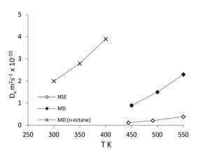
Fig. 9 Comparison of diffusion coefficients of isobutane from NSE ( $\Diamond$ ) and MD ( $\bullet$ ) compared with previous simulations of n-octane diffusion in ref. 51 ( $\times$ ). Reproduced from ref. 59 with permission from the American Chemical Society.
