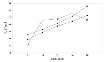
Fig. 5 A plot of the activation energy of diffusion with chain length, for the MD studies at experimental loadings  $(\bullet)$ , <sup>51</sup> QENS studies<sup>47</sup> (\*) and hierarchical simulations  $(\Box)$ . <sup>50</sup> Reproduced from ref. 51 with permission from the PCCP Owner Societies.
