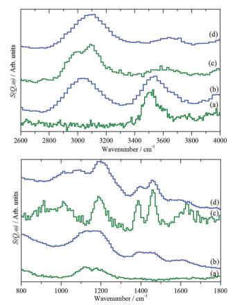
Fig. 15 INS spectra of H-ZSM5 under different conditions for the MTH reaction.<sup>74</sup> (a) The clean catalyst after dehydration at 350 °C and after reaction with methanol at: (b) 350 °C for 1 hour, (c) 350 °C for 3 days and (d) 400 °C for 3 days. Upper part: the C-H and O-H stretch region. Lower part: the fingerprint region.
