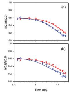
Fig. 7 Comparison between experimental and calculated normalized intermediate scattering functions obtained for isobutane in silicalite-1 at 491 K, for Q=0.2 ( $\nabla$ ) and 0.3 Å $^{-1}$  ( $\diamondsuit$ ). The solid lines are calculated with: (a) a 3D diffusion model, and (b) a 1D diffusion model. Reproduced from ref. 59 with permission from the American Chemical Society.
