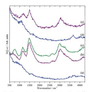
**Fig. 14** INS spectra of methanol loaded in zeolites HY and H-ZSM-5.<sup>65</sup> (a) Clean HY, (b) HY + methanol, (c) solid methanol, (d) clean H-ZSM5 and (e) H-ZSM5 + methanol.
