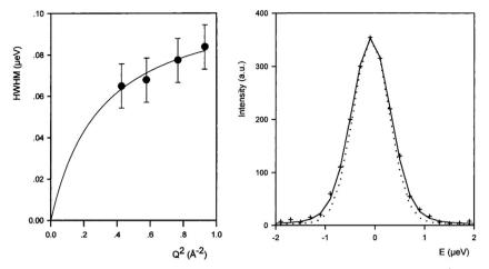
Fig. 6 (left) Broadenings obtained for isobutane in ZSM-5 at 570 K, and QENS spectra obtained at 570 K (Q = 0.87 Å). The dotted line is the resolution function. Reproduced from ref. 55 with permission of the American Chemical Society.
