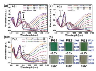
Fig. 3 Spectroelectrochemistry of PG1, PG2 and PG3 film on an ITO-coated glass slide (0.5 cm width) in a monomer-free 0.1 M TBAPF<sub>6</sub>/ACN electrolyte-solvent couple at applied potentials: (a) -0.5 to 0.8 V, (b) -0.3 to 0.9 V, (c) -0.1 to 1.0 V. (d) Photographs and corresponding (Y; x; y) values of PG1, PG2 and PG3 film on an ITO-coated glass slide in the fully neutral and oxidized states.
