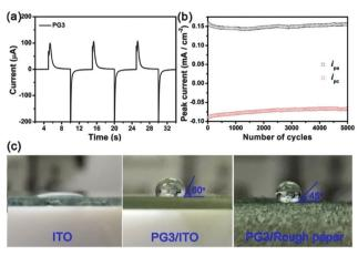
Fig. 4 (a) Chronoamperometry for PG3 with a 5 s delay for each potential (-0.1 V and +0.8 V). (b) Stability of a 600 nm thick PG3 film cycled 5000 times with a scan rate of 100 mV  $s^{-1}$  in 0.1 M TBAPF<sub>6</sub>/ACN: the change in the anodic  $(\Box)$  and cathodic  $(\bigcirc)$  peak currents as a function of number of cycles. (c) Photographs of the water droplet volume of 10 µL on the surface of ITO, PG3/ITO and PG3/rough paper, respectively.
