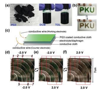
Fig. 5 (a) The appearance of PG3, and in a DCM or TOL solution. Images of the PG3 camouflage fabric with space between each piece, (b) example of the patterned device in neutral and oxidized states, (c) fabric chameleonic electrochromic device cross-section for a typical device used in this study, (d) all pieces 1–7 as the working electrode in their neutral, (e) 1, 2, 3, 4 in neutral and 5, 6, 7 in oxidized, (f) in oxidized states.
