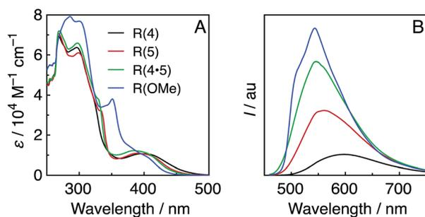
Fig. 1 UV-vis (A) and emission (B) spectra of the Re-rings in DMF under Ar. The emission spectra were corrected to the absorbed photons at  $\lambda_{\text{ex}} = 400$  nm.Table 1 Photophysical properties of **R(X)** measured in DMF or DMA at 25 °C
