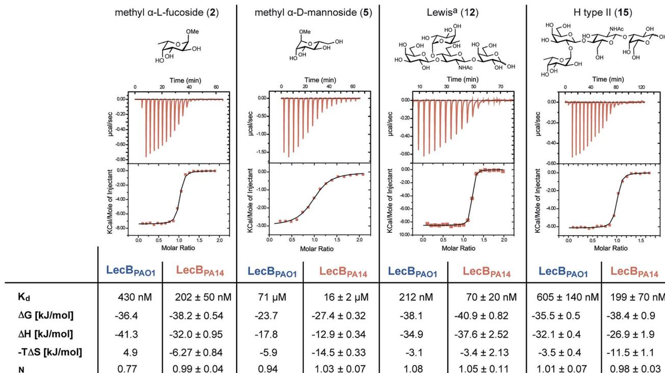
Fig. 4 Isothermal titration calorimetry (ITC) of LecB<sub>PA14</sub> with 2, 5, 12 and 15 and comparison with the titration of 15 against LecB<sub>PAO1</sub> or literature data for 2, 5 and 12 with LecB<sub>PAO1</sub>.<sup>14,30</sup>
