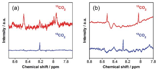
Fig. 7  $^1\text{H}$  NMR spectra of reaction solutions (2 mL) containing RuRu/Ag/TaON (8 mg) in (a)  $\text{H}_2\text{O}$ -MeOH (4 : 1 v/v) and (b)  $\text{H}_2\text{O}$ -iPrOH (4 : 1 v/v) after a 48 h irradiation with visible light ( $\lambda > 400$  nm) under  $^{13}\text{CO}_2$  (red) and  $^{12}\text{CO}_2$  (blue) atmospheres.
