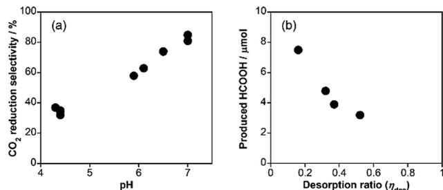
Fig. 4 (a) Selectivity of CO<sub>2</sub> reduction (sel<sub>CO<sub>2</sub></sub>) vs. pH of the reaction solution in the photocatalytic reactions. (b) Produced amount of HCOOH vs. desorption ratio of RuRu (η<sub>des</sub>) by the photocatalytic reactions with various concentration of NaH<sub>2</sub>PO<sub>4</sub> (pH = 4.4).
