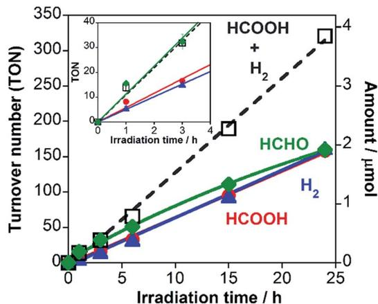
Fig. 6 Time courses of HCOOH (red), H<sub>2</sub> (blue) and HCHO (green) formation along with the sum of HCOOH and H<sub>2</sub> (black broken line) in the photocatalytic reaction: RuRu/Ag/TaON (4 mg) in a H<sub>2</sub>O–MeOH (4 : 1 v/v) mixed solution (4 mL) was irradiated by visible light (λ > 400 nm) under a CO<sub>2</sub> atmosphere. Inset shows enlarged time courses until 4 h irradiation.
