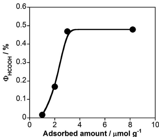
Fig. 5 Relationship between Φ<sub>HCOOH</sub> and loading amount of RuRu in the photocatalytic reaction using RuRu/Ag/TaON (30 mg) and EDTA·2Na (10 mM) in aqueous solution (10 mL) with 400 nm monochromatic light irradiation under a CO<sub>2</sub> atmosphere.
